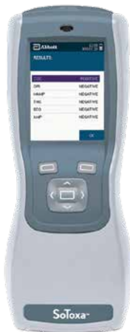
The SoToxa Mobile Test screens for six different classes of drugs in oral fluid. (Image courtesy of Intoximeters.)
