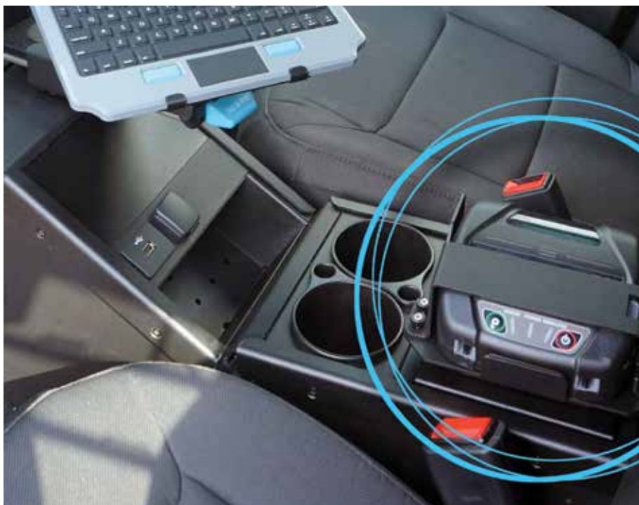
Seiko Instruments' MP-A40 can be mounted in a police vehicle and connected to the vehicle power. (Image courtesy of Seiko Instruments USA, Inc.)
